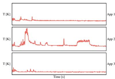
Basic concept thermal task inference side channel
