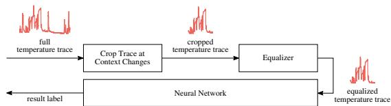
Feasibility study using simple neural networks and augmented thermal data from Dragonboard 810
