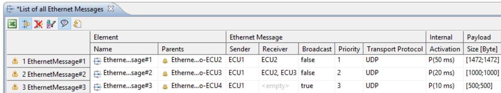
The screenshot shows a software interface titled "List of all Ethernet Messages". The window has a toolbar with various icons at the top. The main area is a table with the following columns: Element, Name, Parents, Sender, Receiver, Broadcast, Priority, Transport Protocol, Activation, and Payload. There are three rows of data in the table:
